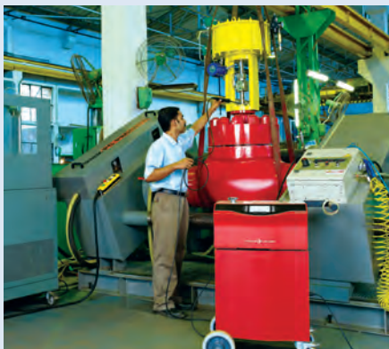
Gland leak measurement for Fugitive Emission testing
