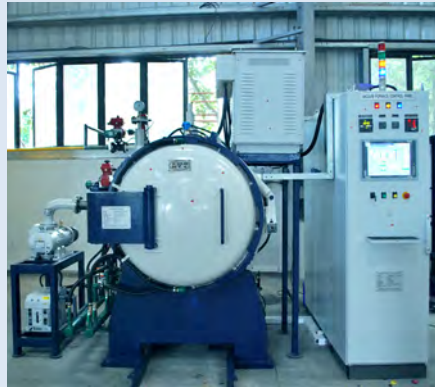
Vacuum Heat Treatment facility
