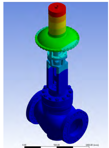
Vibration analysis for seismic qualification
