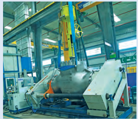
A 32 inch size valve being tested on the High pressure test bench
