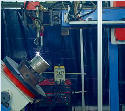
Automatic hard facing process
